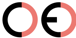
False CE Mark (too far)
